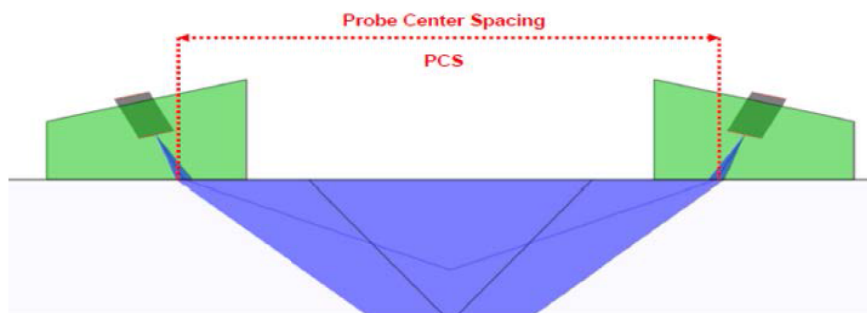
FIG. 5 PCS (Probe Centre spacing)
