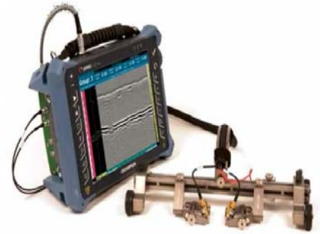
FIG 8 Basic ToFD Instrument
